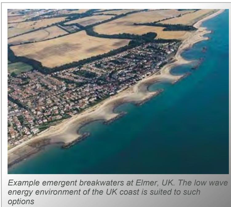
*Example emergent breakwaters at Elmer, UK. The low wave energy environment of the UK coast is suited to such options*
